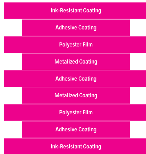
Fig. 4. Nine-layer bag film structure.
